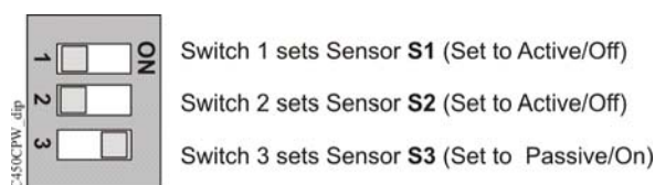
Figure 5: Active/Passive Sensor DIP Switch Block (Set up for Example in Figure 3)
